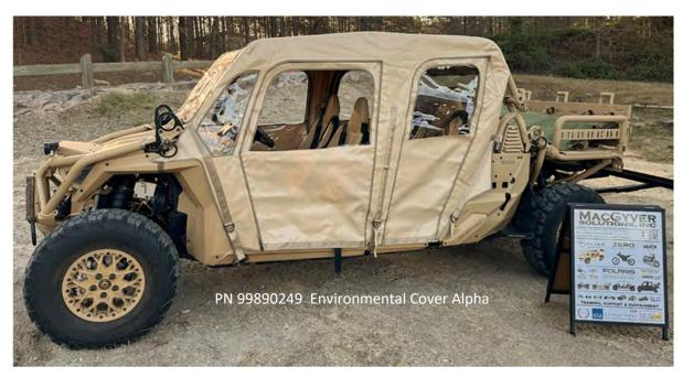
Polaris MRZR-Alpha / Ultra Light Tactical Vehicle -ULTV with Environmental Cover fully installed.
