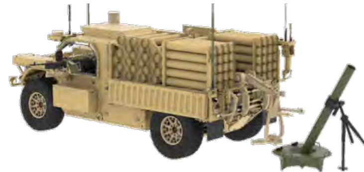
12-Crew Assault Carrier Kit Carries nine seated operators in cargo bed, three in cab
